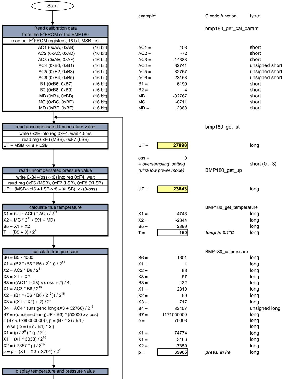
Figure 4: Algorithm for pressure and temperature measurement
