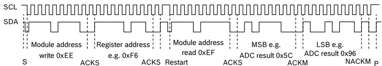
Figure 9: Timing diagram read 16 bit A/D conversion result
