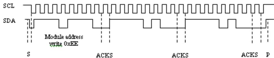
Figure 8: Timing diagram for starting pressure measurement
