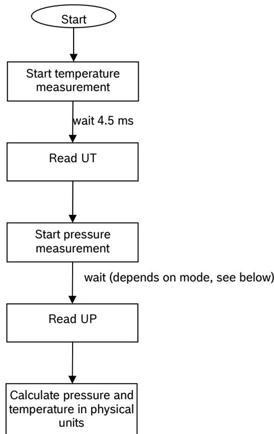
Figure 3: Measurement flow BMP180
